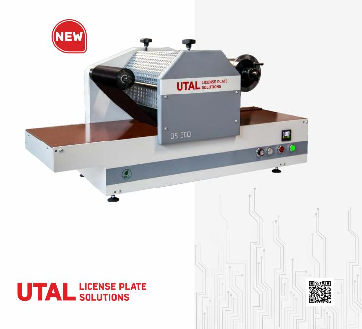
**DS ECO** is an efficient and cost - effective machine designed for the coating of embossed license plates, using hot stamping technology.
